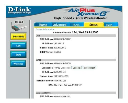
The status and external IP Address of the router are clearly shown in the WAN section.
